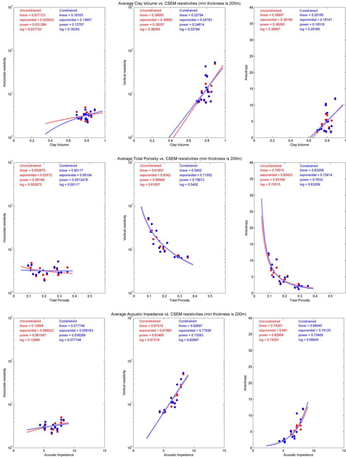
Figure 2: Comparison of unconstrained (red) inversion data and constrained inversion (blue) data for the Sjøhvit overburden sediments. Trends lines shown are the best fit trend. Middle Left – porosity vs. horizontal resistivity, Middle Center - porosity vs. vertical resistivity, Middle Right – porosity vs. anisotropy. Bottom Left – acoustic impedance vs. horizontal resistivity, Bottom Center – acoustic impedance vs. vertical resistivity, Bottom Right – acoustic impedance vs. anisotropy.
