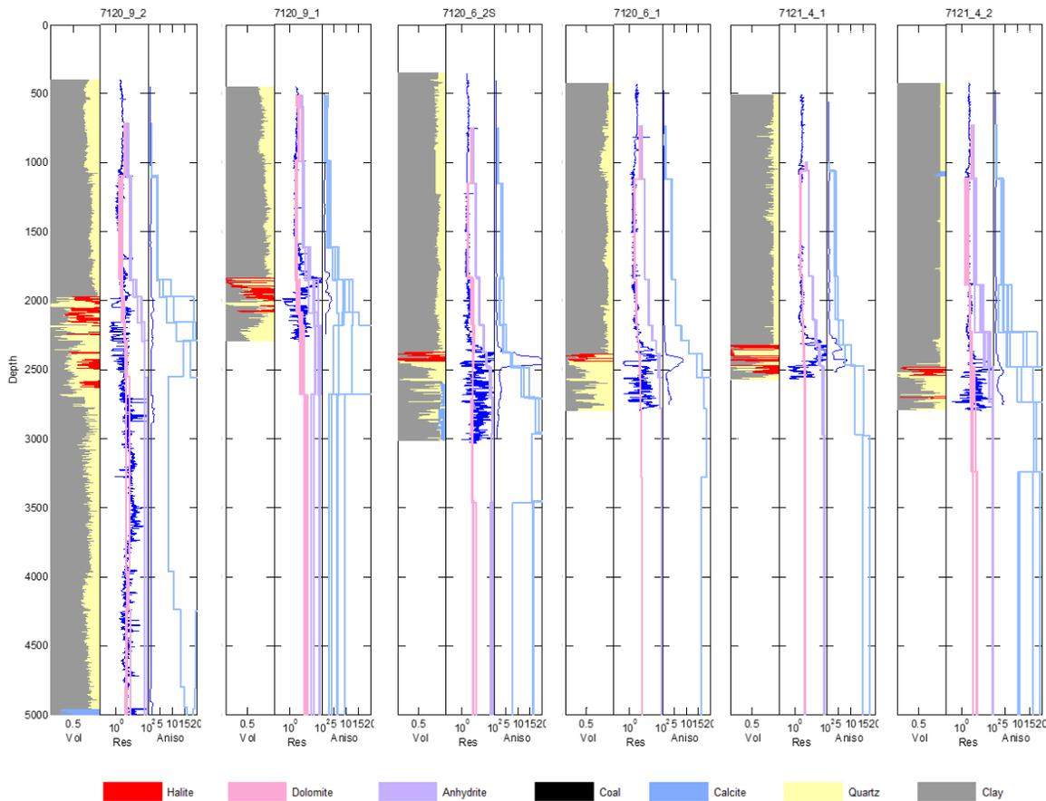
Figure 2: Six Snøhvit wells. Left – sedimentary column with reservoir highed in red. Middle – well log resistivity (thin blue line), CSEM derived horizontal resistivity (pink) and CSEM derived vertical resistivity (purple). Right – anisotropy due to thin layering (dark blue) and CSEM derived anisotropy (light blue).
