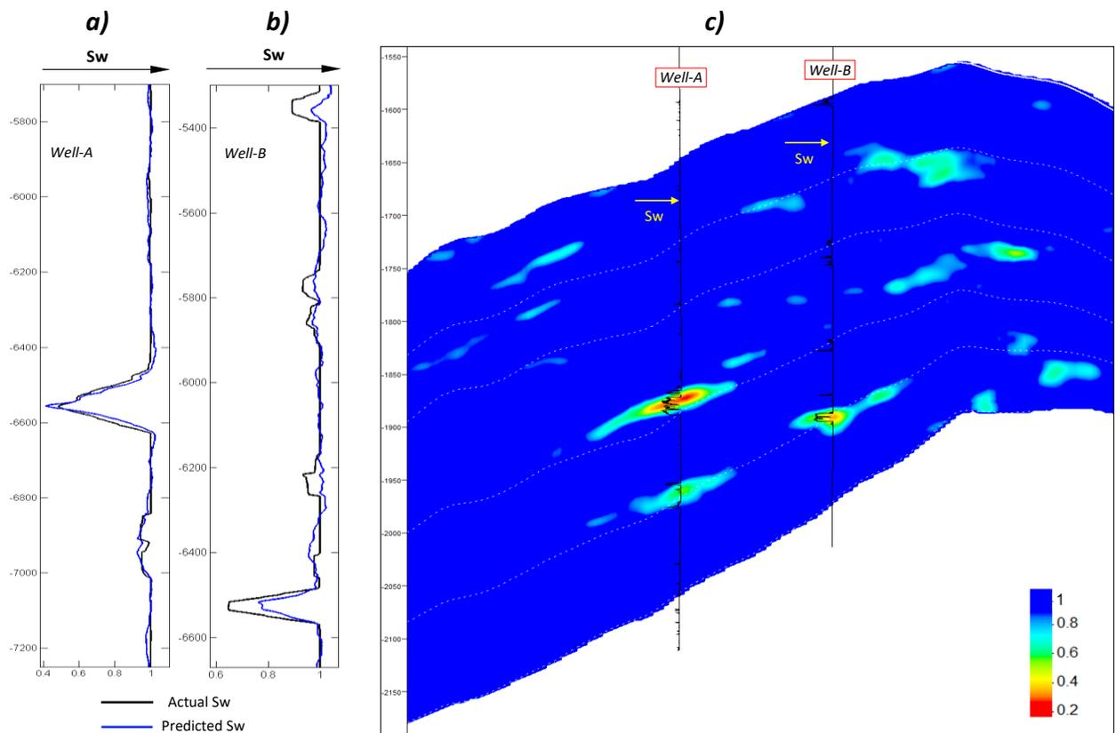
**Figure 2.** a) For well A, comparison between the actual and predicted Sw logs upscaled to seismic resolution. b) For well B (blind test), comparison between the actual and predicted Sw logs, upscaled to seismic resolution, estimated using the transform computed for well A. c) Cross section along the resultant Sw volume along wells A and B (blind well) together with the Sw logs. Notice the good match between the seismic and well-log-derived Sw.
