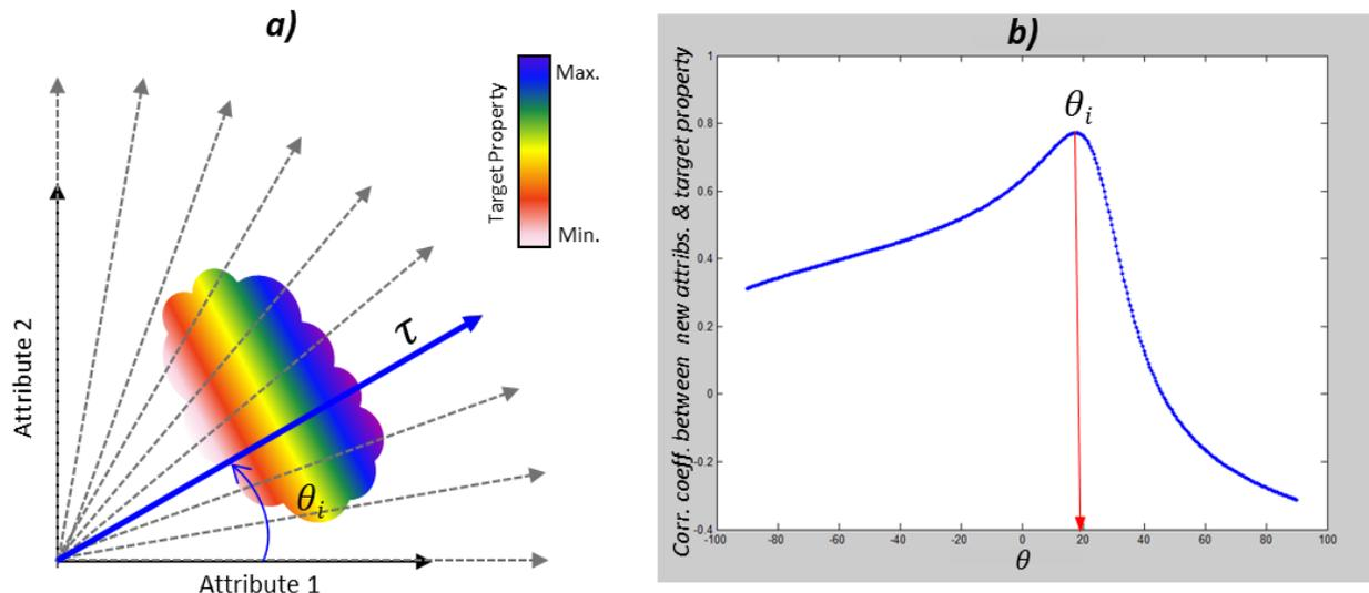
**Figure 1.** a) Sketch of a cross-plot of two attributes color-coded by a target property. Dashed grey lines represent new attributes estimated via axis rotation, and the blue line represents the attribute that shows the maximum correlation coefficient with the target property. b) Example of a cross-plot between the angles of rotation and the correlation coefficients calculated at each of these angles.
