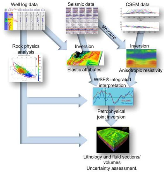
Figure 1: Full PJI workflow, including the electric attribute downscaling (WISE® integrated interpretation).
