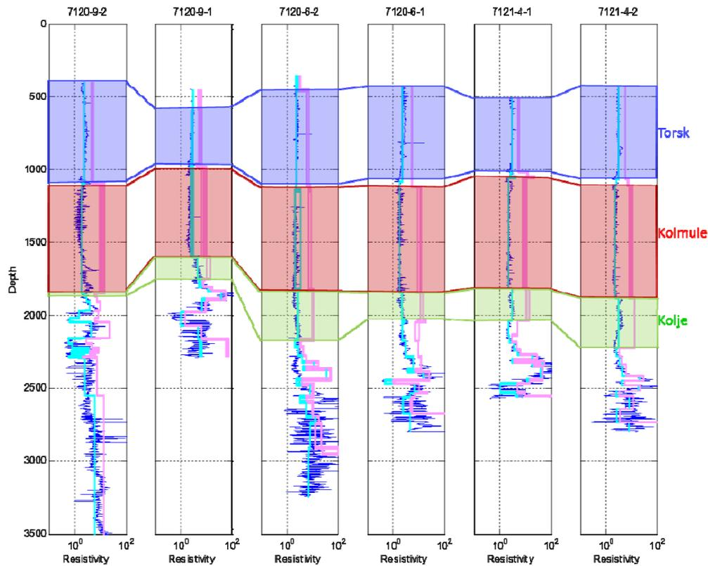
**Figure 1.** Comparison of well log resistivity (blue line), CSEM derived horizontal resistivity (cyan line) and CSEM derived vertical resistivity (pink line) for six wells in the Snøhvit region. Formations used in the trend analysis are highlighted in blue, red and green.
