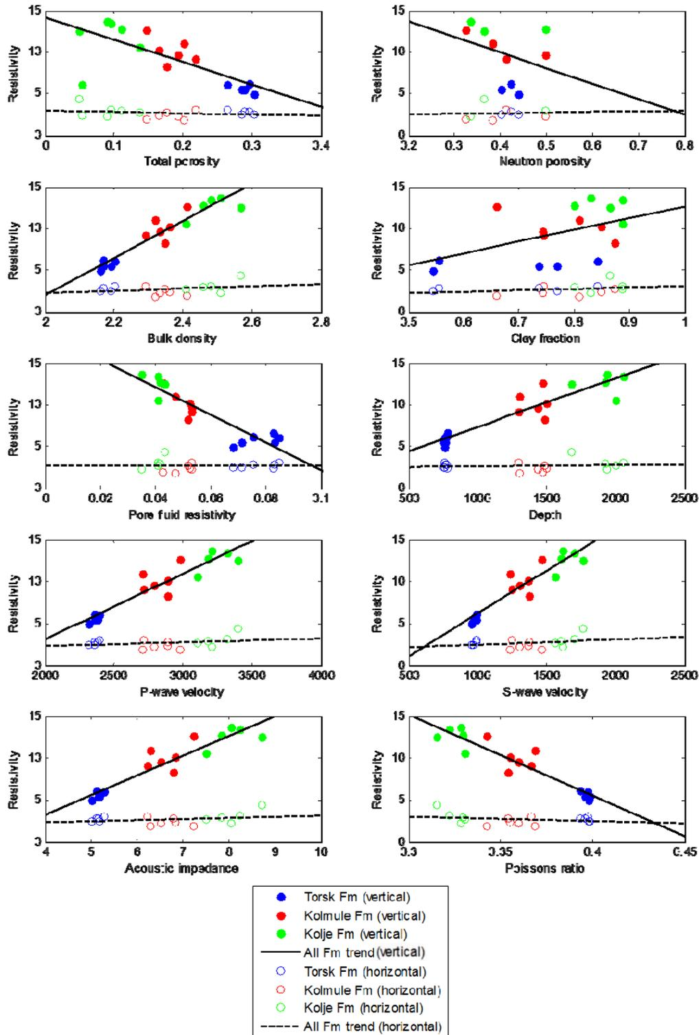
**Figure 2.** Cross plots of vertical resistivity averages (solid circles) and horizontal resistivity averages (open circles) with well log data averages in the Torsk, Kolmule and Kolje formations from the Snøhvit area of the Barents Sea. Trend lines (solid black lines for the vertical resistivities and dashed black lines for the horizontal resistivities) calculated using a linear regression,  $R^2$  values for each plot can be found in Table 1.
